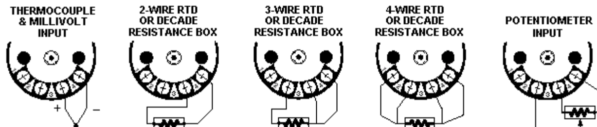
Figure 11. Sensor / input connections for the THZ and TDZ (While terminal placement may differ from unit to unit, all models identical numeric designations)
