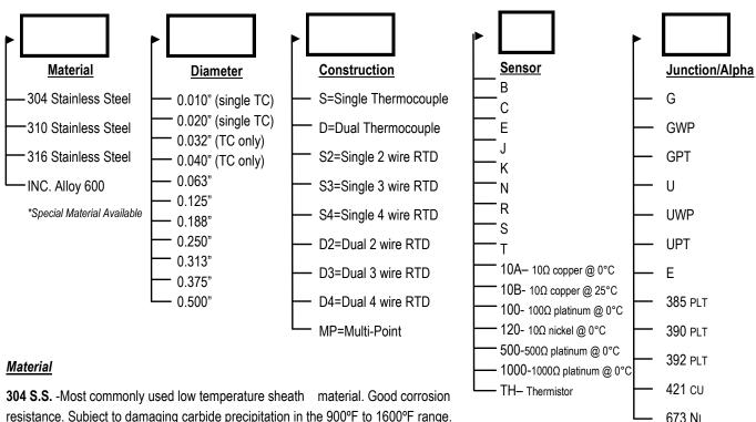
resistance. Subject to damaging carbide precipitation in the 900°F to 1600°F range. Max Temp. 1650°F
